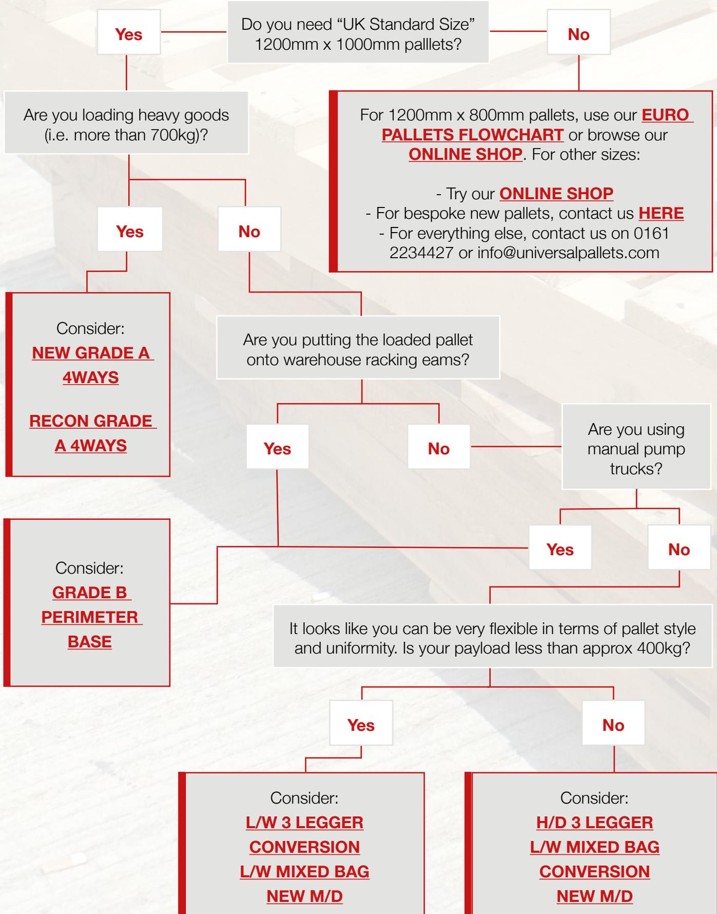
Please note: Payload and stability are greatly affected by things outside of our control, including load stability, loading techniques, whether load is static or dynamic, and temperature. As such, they should always be tested in house to ensure suitability.
